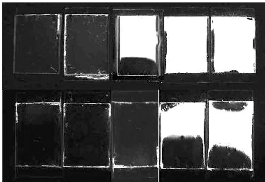
FIGURE 4 Photos of asymmetric cells ( d = 20\ \mu\text{m} ) viewed between a pair of crossed polarizers. The cells are filled with LC 5CB (set (a)) and MJ961180 (set (b)). In each set, the tested PI substrate is treated with plasma beam over 1, 3, 5, 15, and 30 min in static regime.
